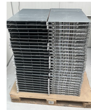
Products are placed on the pallet in such away that they do not fall outside the pallet edge
