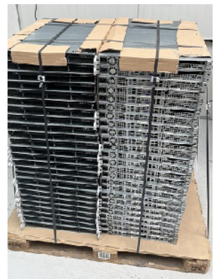
Products are secured to the pallet with tension straps. To protect the corners, they are protected with cardboard profiles.
