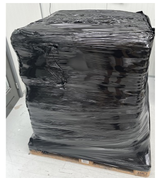
The whole thing is then wrapped in a layer of sealing foil. This provides protection and is splash-proof, so the products arrive dry.
